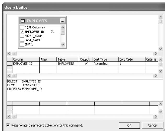
**Figure 2-24.** Setting the properties in the Query Builder
