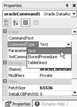
**Figure 2-3.** *Setting the CommandType property at design time*
