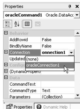
**Figure 2-2.** Setting the `Connection` property using the Visual Studio Properties window
