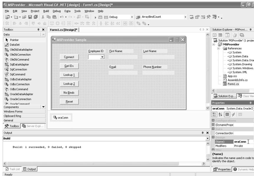
Figure 2-19. Creating the OracleConnection object on the form
