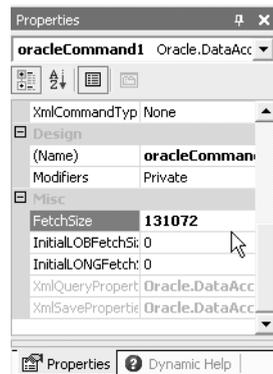
**Figure 2-6.** Setting the `FetchSize` property to 128K in the Properties window
